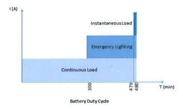
13. Emergency lighting system shall be installed at the GIS building in case of normal station service fails. The said emergency lighting system be activated and capable of generating illumination level of at least 150 lux for at least 3 hours.
