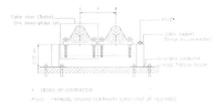
The cable supporting structure shall be made of stainless steel, aluminum alloy or galvanized steel. The contractor shall design, supply and install the cable supporting structures that are suitable for cable cleat and cable system installation, and their grounding.
