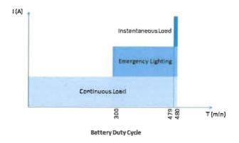
2.4 Emergency lighting system shall be installed at the Control building and Switchgear building in case of normal station service fails. The said emergency lighting system is activated and capable of generating illumination level of at least 150 lux for at least 3 hours.
