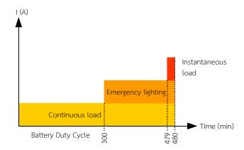
2.4 Emergency lighting system shall be installed at the control building,230 kV GIS building and 115 kV GIS building in case of normal station service fails. The said emergency lighting system is activated and capable of generating illumination level of at least 150 LUX for at least 3 hours.
