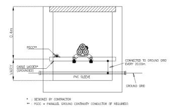
The cable support structure shall be made of stainless steel, aluminum alloy or galvanized steel. The contractor shall design, supply and install the cable supporting structures that are suitable for cable cleats and cable system installation and their grounding. The ground shielding shall be directly connected to ground grid and shall not be connected with other equipment's grounding material before connecting to ground grid.
