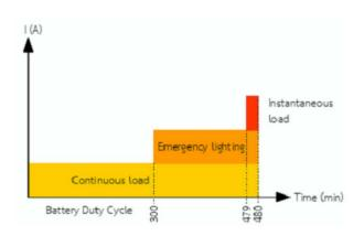
2.4 Emergency lighting system shall be installed at the 115kV GIS building, control building and 33kV switchgear building in case of normal station service fails. The
