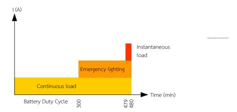
2.4 Emergency lighting system shall be installed at the control building,230 kV GIS building and 115 kV GIS building in case of normal station service fails. The said emergency lighting system is activated and capable of generating illumination level of at least 150 LUX for at least 3 hours.
