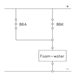
3.11 Signals of indoor fire protection system of each room and signals of outdoor fire protection system of each transformer shall be sent to local CCS, GCC, RCC, and NCC as following details;
