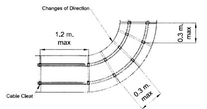
For 22 kV system the calculation of forces caused by short-circuit currents, the peak short circuit current shall be 62.5 kA, trefoil formation. The cable supporting structure shall be made of stainless steel, aluminum alloy or galvanized steel. The contractor shall design, supply and install the cable supporting structures that are suitable for cable cleat and cable system installation, and their grounding.
